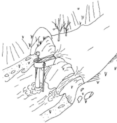
Dams have both advantages and dis-advantages. If used in a village setting they can provide additional uses as a fish pond and washing area. The dam wall may support a row of PowerPal generators so that several families can have access to electricity. If the village works together to build the dam the time and construction costs are lower. Dams are less likely to be effected by flooding if diversion channels are adequate, so PowerPal can be used effectively during the rainy season.
